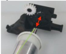
**15.** Make sure the end of the tension roller is aligned as shown:
